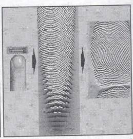
Figure 2.12. As the user sweeps her finger on the sensor, the sensor delivers new image slices, which are combined into a two-dimensional image.
