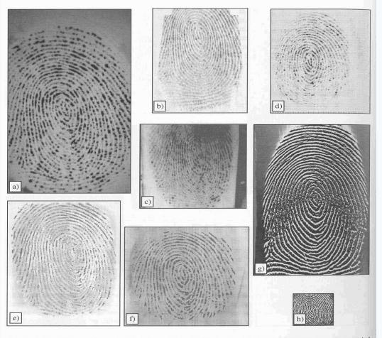
Figure 2.15. Fingerprint images of the same dry finger as acquired by different commercial scanners. Images are reported with right proportions: a) Biometrika FX2000, b) Digital Persona UareU2000, c) Identix DFR200, d) Ethentica TactilSense T-FPM, e) ST-Microelectronics TouchChip TCS1AD, f) Veridicom FPS110, g) Atmel FingerChip AT77C101B, h) Authentec AES4000.
