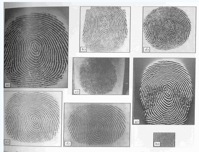
igure 2.14. Fingerprint images of the same finger with ideal skin condition as acquired by diferent commercial scanners. Images are reported with right proportions: a) Biometrika FX2000, b) Digital Persona UareU2000, c) Identix DFR200, d) Ethentica TactilSense T-FPM, e) STdicroelectronics TouchChip TCS1AD, f) Veridicom FPS110, g) Atmel FingerChip AT77C101B, b) Authentec AES4000.
