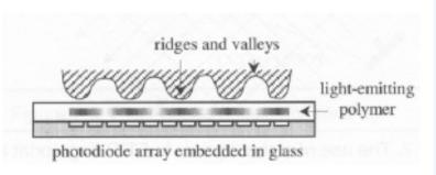
Electro-optical fingerprint sensor
