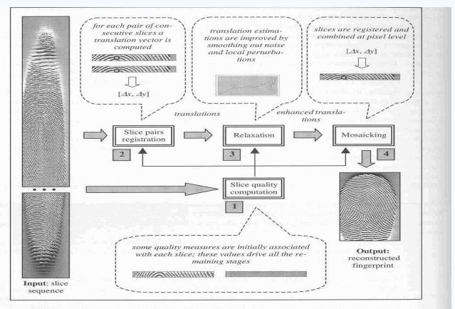
Figure 2.13. An algorithm for fingerprint reconstruction from slices. All the steps are performed sequentially on the whole set of slices. The output of the slice pair registration is a set of translation estimates that are globally enhanced by the relaxation step. These improved estimates drive the mosaicking phase in order to reconstruct the whole fingerprint image.
