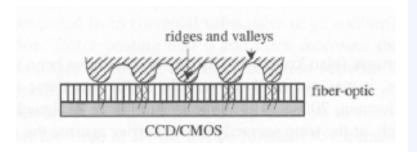
Sensor based on optical fibers
