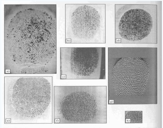
Figure 2.17. Fingerprint images of the same poor quality finger as acquired by different commercial scanners. Images are reported with right proportions: a) Biometrika FX2000, b) Digital Persona UareU2000, c) Identix DFR200, d) Ethentica TactilSense T-FPM, e) ST-Microelectronics TouchChip TCS1AD, f) Veridicom FPS110, g) Atmel FingerChip AT77C101B, h) Authentec AES4000.
