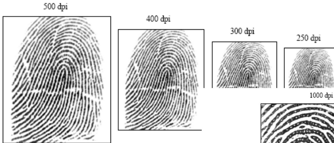
Figure 2.15. The fingerprint on the left, acquired at 500 dpi, is compared with lower resolutions: 400, 300, and 250 dpi, respectively.
