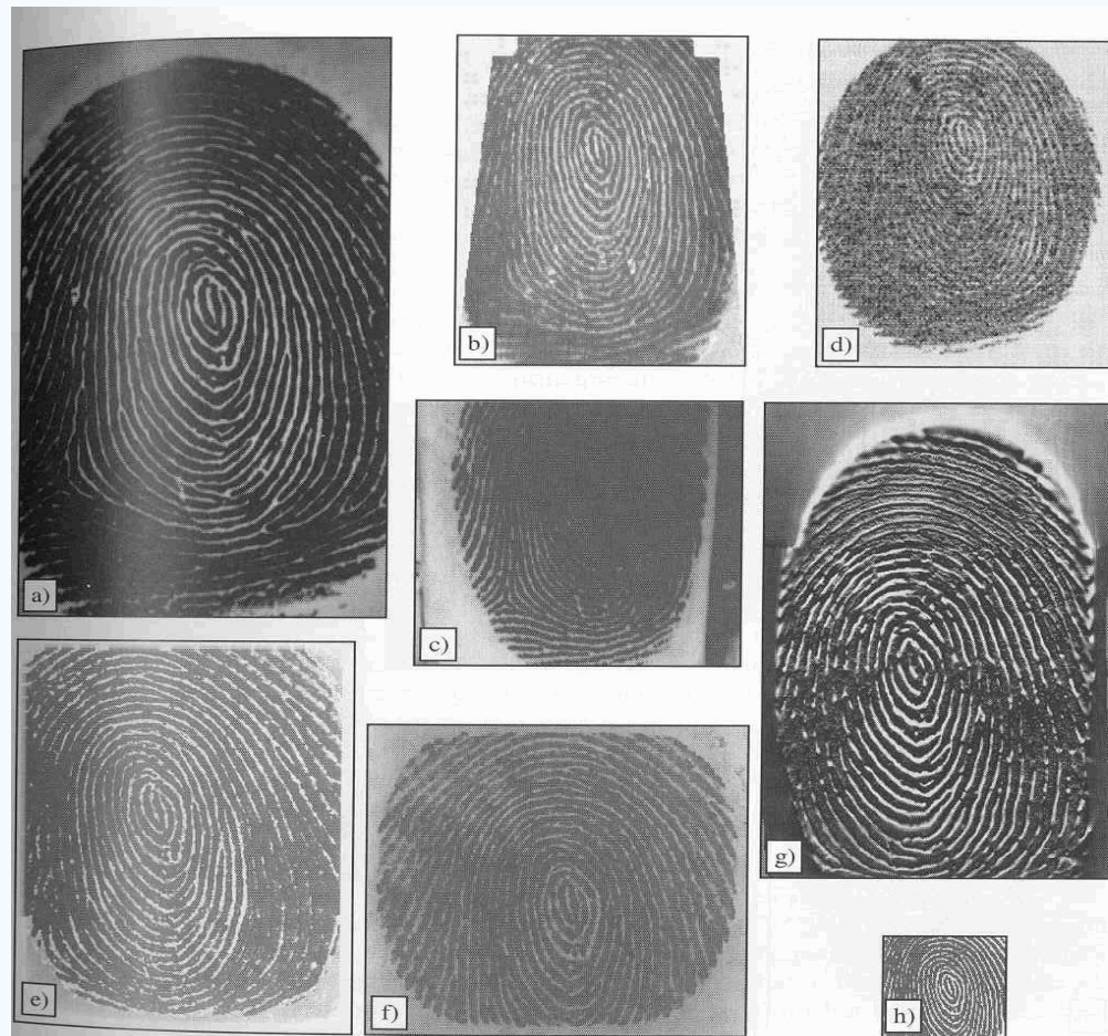
Figure 2.16. Fingerprint images of the same wet finger as acquired by different commercial scanners. Images are reported with right proportions: a) Biometrika FX2000, b) Digital Persona UareU2000, c) Identix DFR200, d) Ethentica TactilSense T-FPM, e) ST-Microelectronics TouchChip TCS1AD, f) Veridicom FPS110, g) Atmel FingerChip AT77C101B, h) Authentec AES4000.
