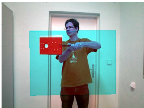
Figure 4: An example of the calibration result. Pixels corresponding to the thermo-camera field-of-view are colored according to their temperature (blue is cold, red is hot).
