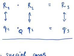
can be represented by  $\vec{q}_{21}$ . Let us investigate how to obtain  $\vec{q}_{21}$  from  $\vec{q}_1$  and  $\vec{q}_2$ . We shall use Equation 1.76 to relate R<sub>1</sub> to  $\vec{q}_1$  and R<sub>2</sub> to  $\vec{q}_1$ , then evaluate R<sub>21</sub> = R<sub>2</sub> R<sub>1</sub> and recover  $\vec{q}_{21}$  from R<sub>21</sub>. We use Equation 1.23 to write
