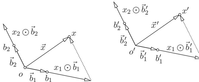
Figure 4.6: Two sets of bound vectors  $A_o$  and  $A_{o'}$ . Coordinates of  $\vec{x}$  w.r.t.  $[\vec{b}_1, \vec{b}_2]$  are equal to coordinates of  $\vec{x}'$  w.r.t.  $[\vec{b}'_1, \vec{b}'_2]$ .
