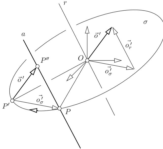
Figure 7.2: Axis  $a$  of motion is parallel to the axis of rotation  $r$  and intersects the perpendicular plane  $\sigma$  passing through the origin  $O$  at a point  $P$ , which is first rotated in  $\sigma$  away from  $a$  to  $P'$  and then returned back to  $P''$  on  $a$  by translation  $\vec{\delta}'$ . Point  $P$  is determined by the component  $\vec{\delta}'_{\sigma}$  of  $\vec{\delta}'$ , which is in the plane  $\sigma$ .
