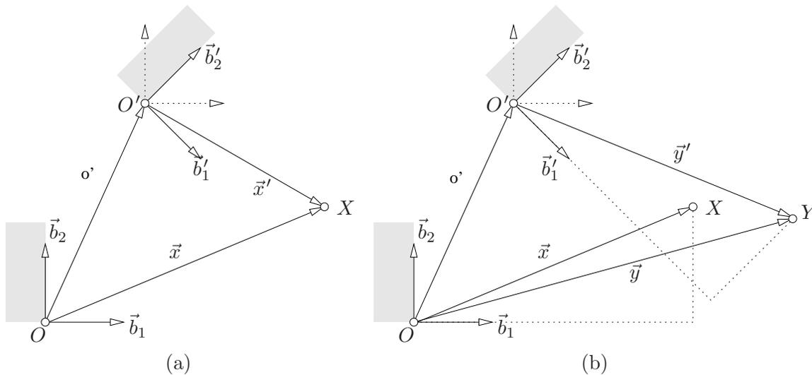
Figure 5.1: Representation of motion. (a) Alias representation: Point  $X$  is represented in two coordinate systems. (b) Alibi representation: Point  $X$  move together with the coordinate system into point  $Y$ .
