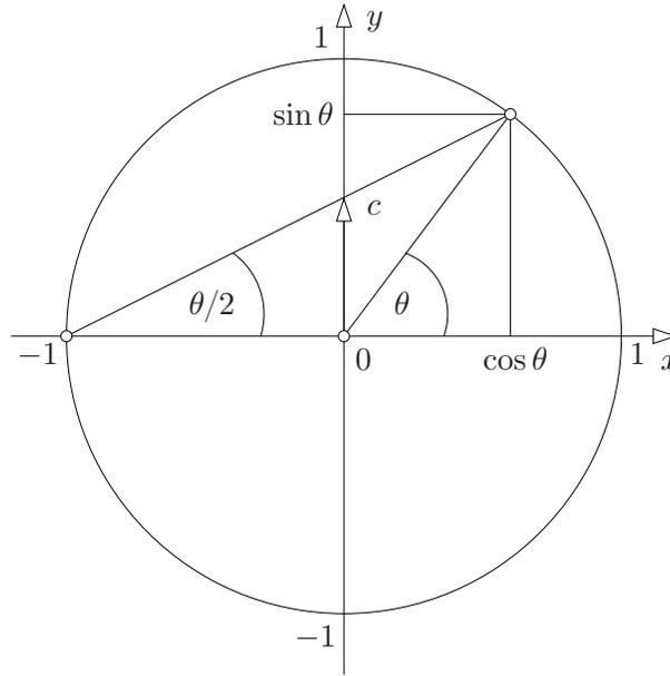
Figure 8.2: Cayley transform parameterization of two-dimensional rotations.
