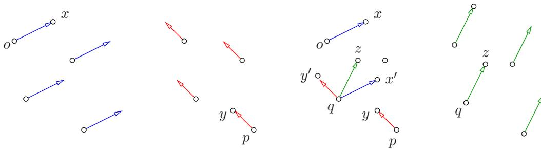
Figure 4.8: Free vector  $A_{(o,x)}$  is added to free vector  $A_{(p,y)}$  by translating  $(o, x)$  to  $(q, x')$  and  $(p, y)$  to  $(q, y')$ , adding bound vectors  $(q, z) = (q, x') \oplus (q, y')$  and setting  $A_{(o,x)} \boxplus A_{(p,y)} = A_{(q,z)}$
