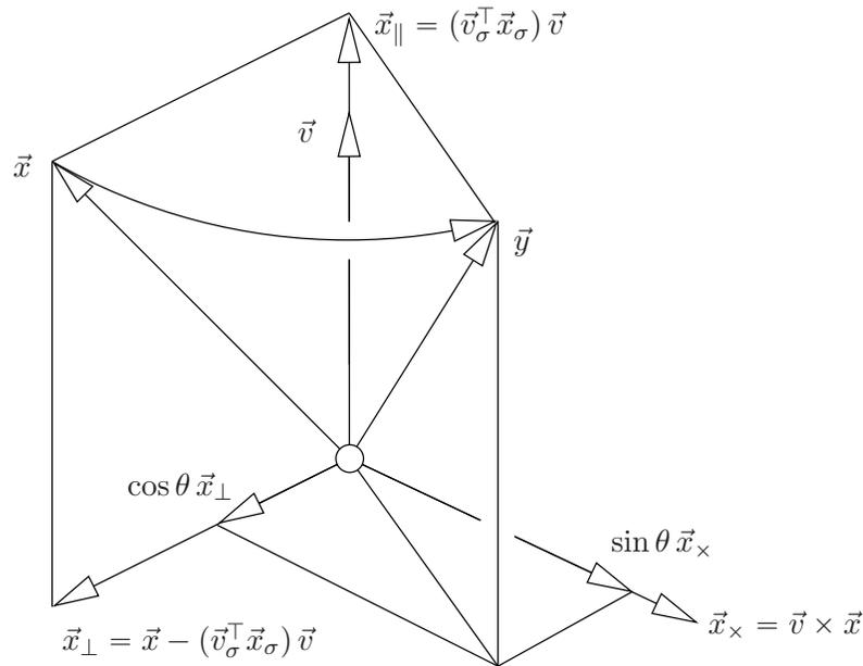
Figure 8.1: Vector  $\vec{y}$  is obtained by rotating vector  $\vec{x}$  by angle  $\theta$  around the rotation axis given by unit vector  $\vec{v}$ . Vector  $\vec{y}$  can be written as a linear combination of an orthogonal basis  $[\vec{x} - (\vec{v}^\top \vec{x}_\sigma) \vec{v}, \vec{v} \times \vec{x}, (\vec{v}^\top \vec{x}_\sigma) \vec{v}]$ .
